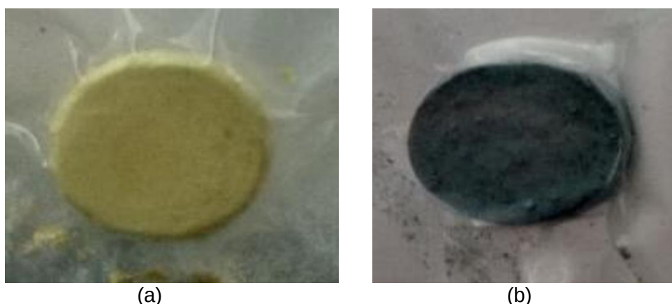
Gambar 5 (a) Tablet indikator kontrol (b) Tablet indikator terpapar gas etilen
